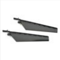
Upper Main Blade Set (1 pair): BMCX, BMCXT (EFLH2221)
